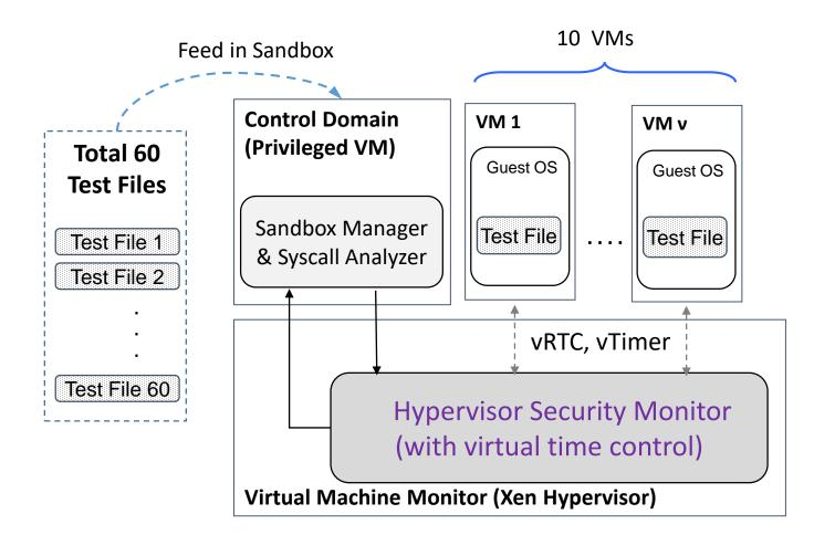
The sandbox system had executed the ten VMs in parallel in the VTC environment until all 60 test files were analyzed
